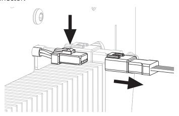
Step 4: Connect each power connector on new fan assembly.
