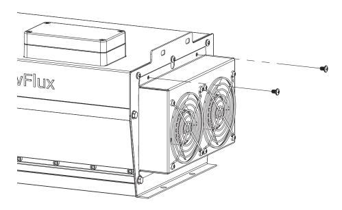
Step 2: With two hands, draw fan assembly upward until fan assembly stops, then draw fan assembly straight outward away from FluxScale.
