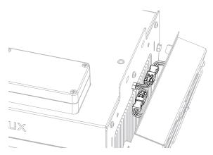
Step 6: Carefully position new fan assembly against FluxScale end plate, taking care to ensure all wires are tucked into fan assembly. Insert mounting tabs into end plate and slide fan assembly downward to lock its position. Install two 8-32 Philips head screws to secure new fan assembly.
